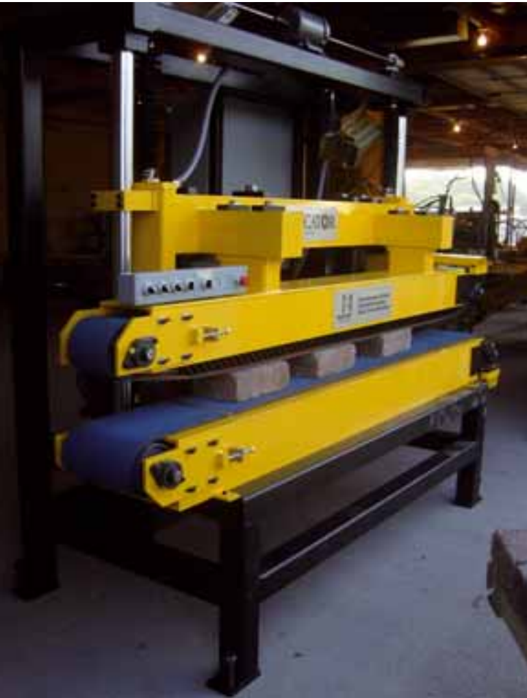
The Rusticator E.D.S. is an in-line concrete block distressing or “anti-queing” machine
